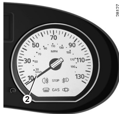
Speedometer 2 Dual speed scale (miles per hour and km per hour) (depending on vehicle)
