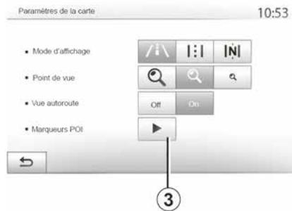
This function allows you to adjust the basic zoom and tilt levels to your needs. Press the required zoom from three available levels.
