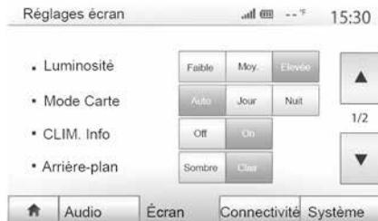
To access the multimedia system settings from the home screen, press "Settings" then select a section at the bottom of the screen.
