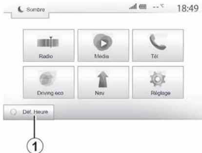
When fitted, this function can be used to program the engine to start remotely in order to heat or ventilate the passenger compartment up to 24 hours before the vehicle is used.
