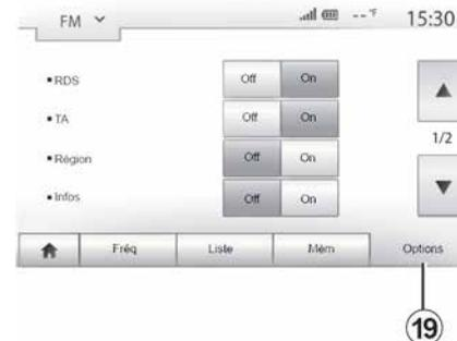
Display the settings menu by pressing **19**. You can activate or deactivate functions by pressing "On" or "Off" (the configuration menu changes according to the band).
