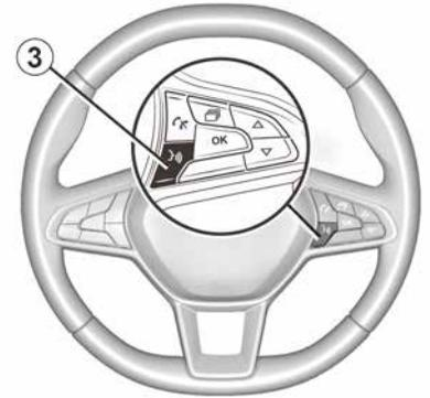
Once the "Android Auto™" application or the "CarPlay™" service is activated, you can use the voice recognition button in your vehicle to activate some of your smartphone functions by voice. To do this, press button **3** on the steering wheel of your vehicle ➔ 61.
