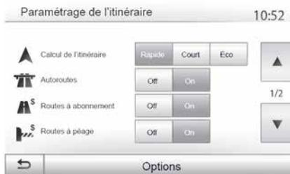
– "Eco": this mode produces a compromise between fast and short routing modes. If you can save a certain distance by travelling for slightly longer time in exchange, it will do just that. The resulting route might be shorter than the fast variant, but not significantly slower.
