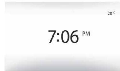
The standby screen mode allows the display screen to be switched off. When in standby clock mode, the radio or guidance system does not operate. The standby screen displays the time and exterior temperature. Briefly press **A** to activate/deactivate the standby screen.
