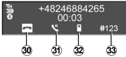
To accept an incoming call, press button **10** on the audio system front panel, or **18**, **21** or **26** on the steering column control, or **28** on the steering wheel.
