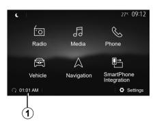
When fitted, this function lets you programme the engine to start remotely, in order to heat or ventilate the passenger compartment up to 24 hours before using the vehicle.
