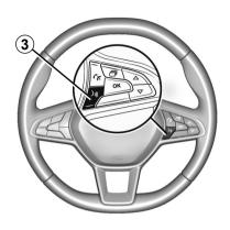
Once the "Android Auto™" application or the "CarPlay™" service is activated, you can use the voice recognition button in your vehicle to activate some of your smartphone functions by voice. To do this, press button 3 on the steering wheel of your vehicle (for more information, refer to the section on "Using voice recognition").
