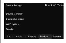
From the welcome screen, select "Settings" > "Devices" > "Device Manager", you can manage the devices connected to your multimedia system at any time.
