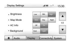
To access the multimedia system settings from the welcome screen, press "Setting", then select a section at the bottom of the screen.
