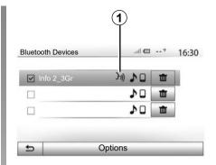
**Note:** the mark **1** on the "Settings" > "Connectivity" then "View Bluetooth device list" menu indicates that your smartphone voice recognition is compatible with the multimedia system.
