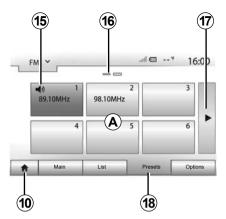
The names of the radio stations that do not use RDS will not appear on the screen. Only their frequency is displayed and sorted at the end of the list.
