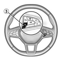
Once the "Android Auto<sup>™</sup>" application or the "CarPlay<sup>™</sup>" service is activated, you can use the voice recognition button in your vehicle to activate some of your smartphone functions by voice. To do this, press button **3** on the steering wheel of your vehicle (for more information, refer to the section on "Using voice recognition"). Note:
