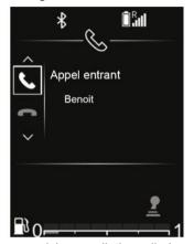
When receiving a call, the caller's number is displayed on the audio system screen (this function depends on the options you have subscribed to with your telephone service provider). If the caller's number is in one of the memories, the name of the caller is displayed instead of the number. If the caller's number cannot be displayed, the "Private number"
