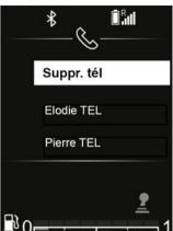
Unpairing allows a phone to be deleted from the audio system memory.
