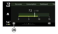
This function displays the current fuel consumption compared to the average consumption of your vehicle.
