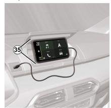
Depending on the equipment, while using the "Dacia Media Control" app your phone can be attached to the centre console thanks to its ergonomic shape **35**.
